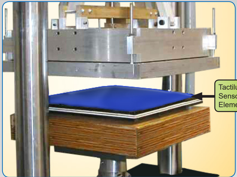
Tactilus® sensor element placed on a lamination press
